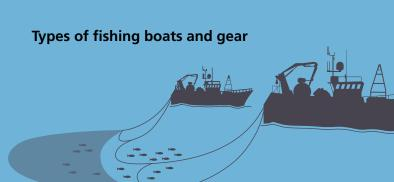
Pair trawler Pair trawlers work as a team to efficiently cover a large amount of water with the minimum amount of fuel. Each boat is connected to one side of the net working as a team. At the end of the trawl the rope from one boat is passed to the other who pulls in the net. This type of fishing mainly targets species such as cod, haddock, and hake.
