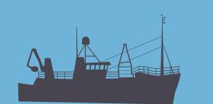
Creel boats They use static gear such as lobster pots that are baited and dropped along the seabed and collected at a later time. These boats are often dual purpose and are also used to catch mackerel in season using a long line - this is known as jigging.
