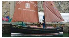
Built by James Weir, Arbroath, the Isabella was launched on the 15th September 1890. With an overall length of 45 feet, 13 feet 9 inches beam and a draught of 6 feet. She was powered by two big lug sails, a jib and five oars and was intended for line and drift-net fishing. In 1997 the Wick Society bought the Isabella Fortuna from Hobson Rankin and since that date enthusiastic volunteers have been engaged on a continuous programme of renewal and restoration.
